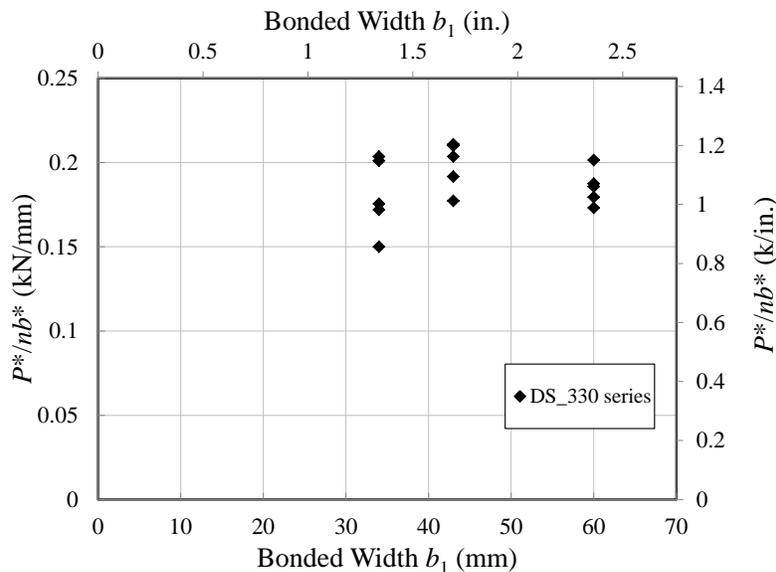
Figure 3.5. Normalized load versus bonded width
