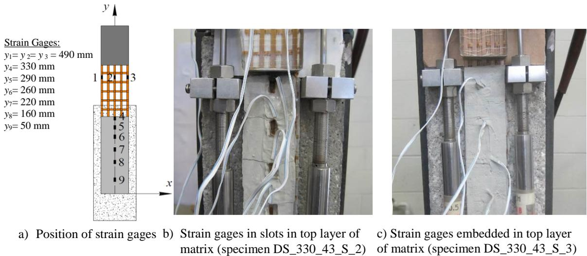
Figure 2.3. Strain gage position and application
