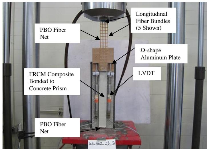
Figure 2.2. Photo of specimen DS\_330\_43\_3
