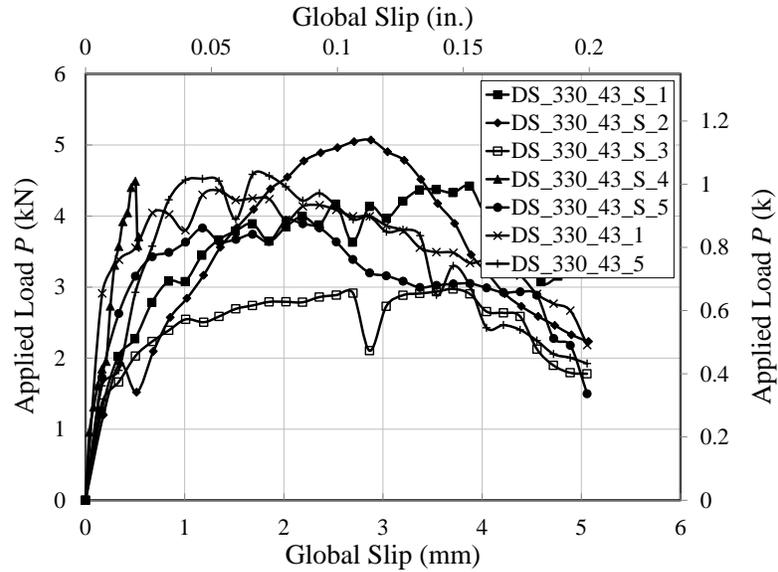
Figure 3.2. Load slip responses for specimens with strain gages
