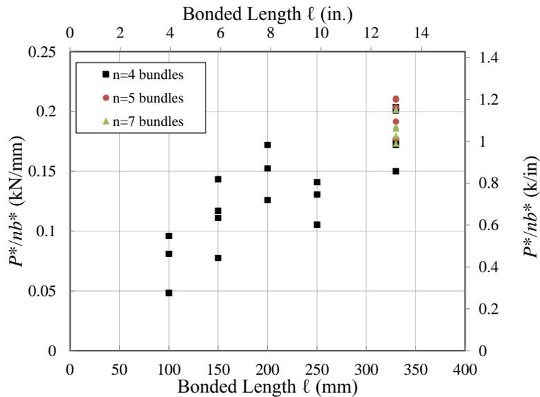
Figure 3.4. Normalized load versus bonded length
