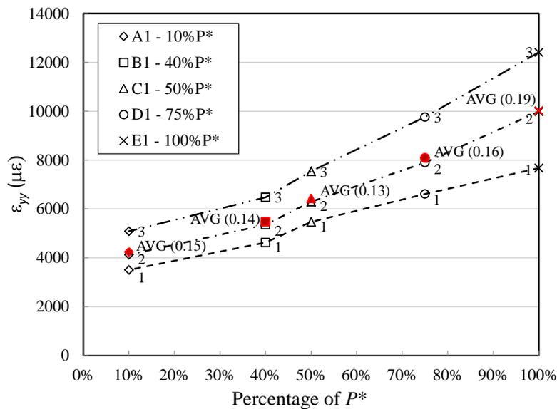
Figure 3.6. Strain in central and edge bundles outside the bonded region of specimen DS\_330\_43\_S\_1
