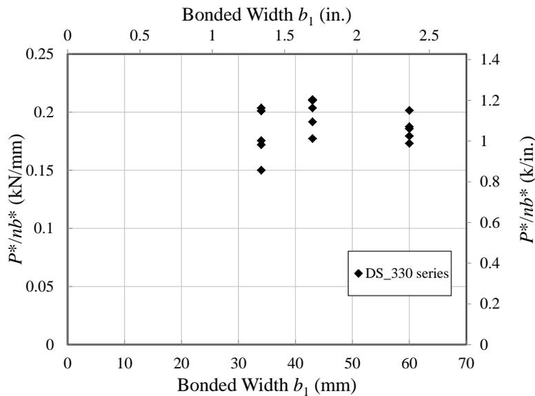
Figure 3.5. Normalized load versus bonded width
