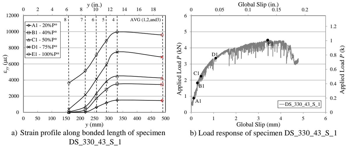
Figure 3.7. Strain profile along bonded length of specimen DS\_330\_43\_S\_1
