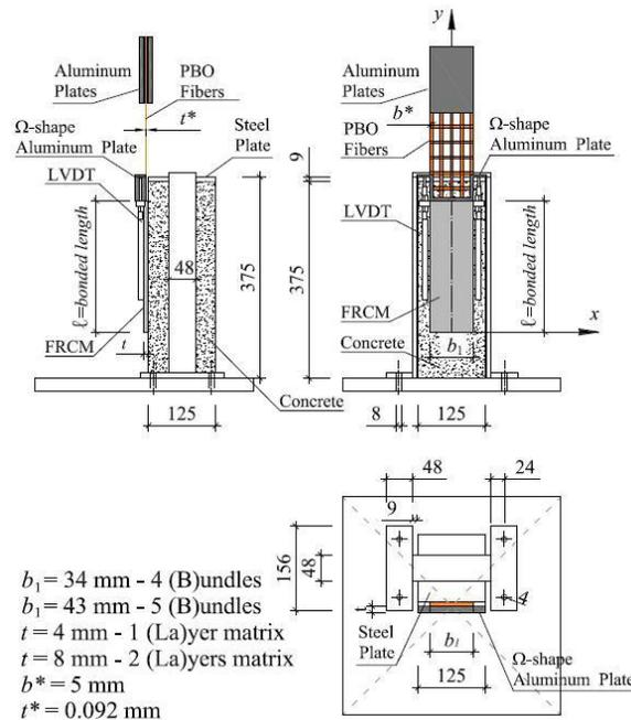
Figure 2.1. Test setup (dimensions in mm; 1 mm = 0.0394 in.)
