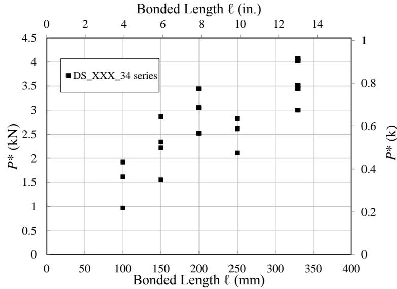
Figure 3.3. Load versus bonded length
